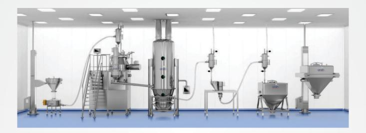
Anish Granulation Line is a complete process line involving stepwise operation, wherein the final product/ output is compressible granules of required size.
