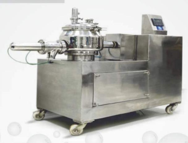
Anish Rapid Mixer Granulator is used for tablet formulation by wet Granulation to reduce processing time, homogeneous mixing, and uniformity of Granules size
